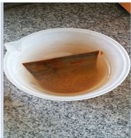
FIGURE 7: SHOWS STAINLESS STEEL PLATE AFTER 24 HOURS OF BIOFILM FORMATION:
